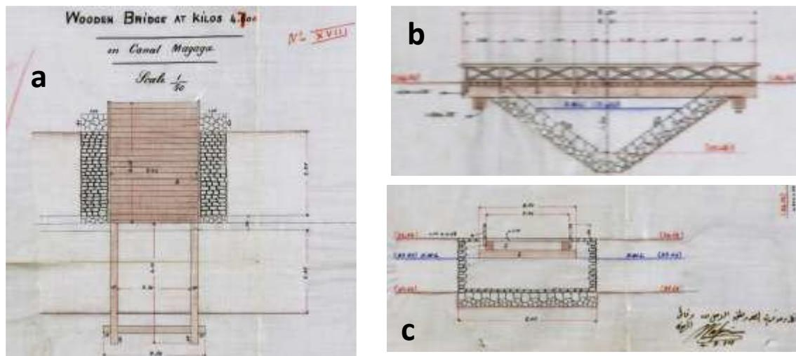
Figure (12) a. plan of Magaga Bridge at kilometre 4.700, b. Longitudinal section of Magaga Bridge, c. end elevation of Magaga Bridge (Documents of Magaga Canal Bridge, code no. 4003-030479).
