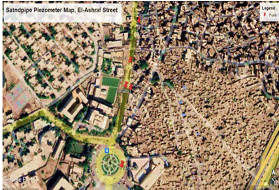
Figure 6. Locations of the piezometers (Marked with the red signs)
